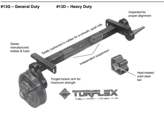
CAUTION: Triple axles assemblies are not recommended for Torflex® axles.
